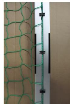
Pull the cord through each net meshes and fix it on both net hoops, if necessary lead it through the bore in the net hoop.
