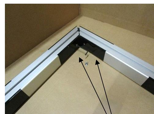
4. screw hexagon socket screws M8 x 20mm slightly
