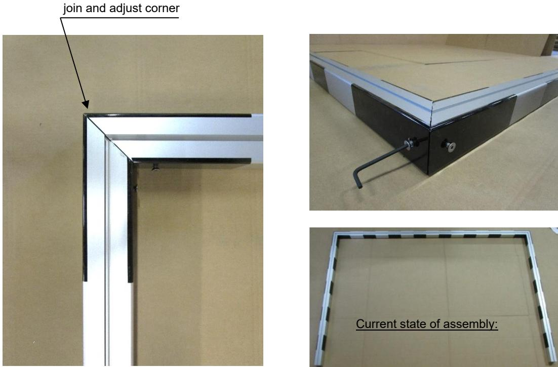
Advice: Due to production tolerances of the aluminium cast corner joints problems during adjustment of corners may possibly occur. Then shorten the stamps in the uprights with a flat file.
