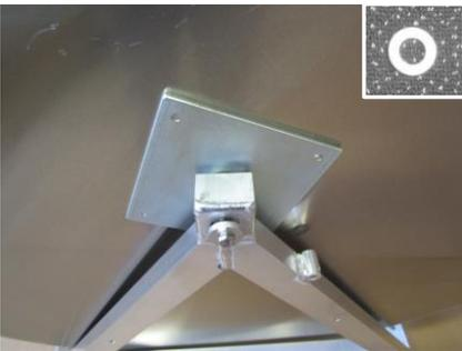
Stick 1 washer  $\varnothing$  outside 28mm, DIN 125-1 on the provided screwing device and screw it firmly into the thread of the plug plate. Make sure that the reel can move freely.
