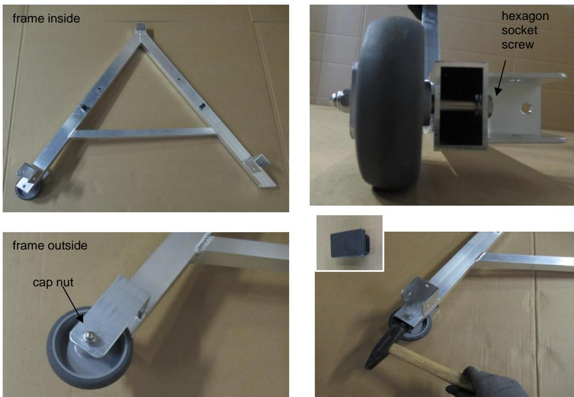
Fix plastic plates rectangular in bottom holes of frame side parts. Use a hammer/mallet if necessary.
