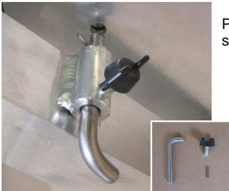
Push from the outside composing stick  $\varnothing$  9mm through the sleeve hole and fix it with a wing bolt M8 x 16.
