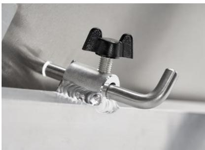
To lock the reel unlock wing bolt, push composing stick into the hole at the round side part and then tighten wing bolt.
