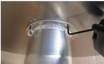
**Attention: The reel tube has to be protected against slipping and overturning before the following assembly!**
