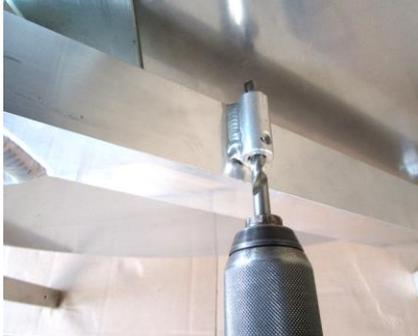
A sleeve with thread M8 is welded on one of the reel supports. Bore a hole for the lock through the sleeve with drill  $\varnothing$  9.5 mm at any position in the round side part.
