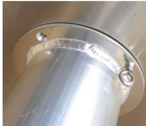
To fix the plug plate stick threaded eye from the reel tube side through the flat hole of reel tube flange and side part (see left picture) and screw it slightly into the plate.
