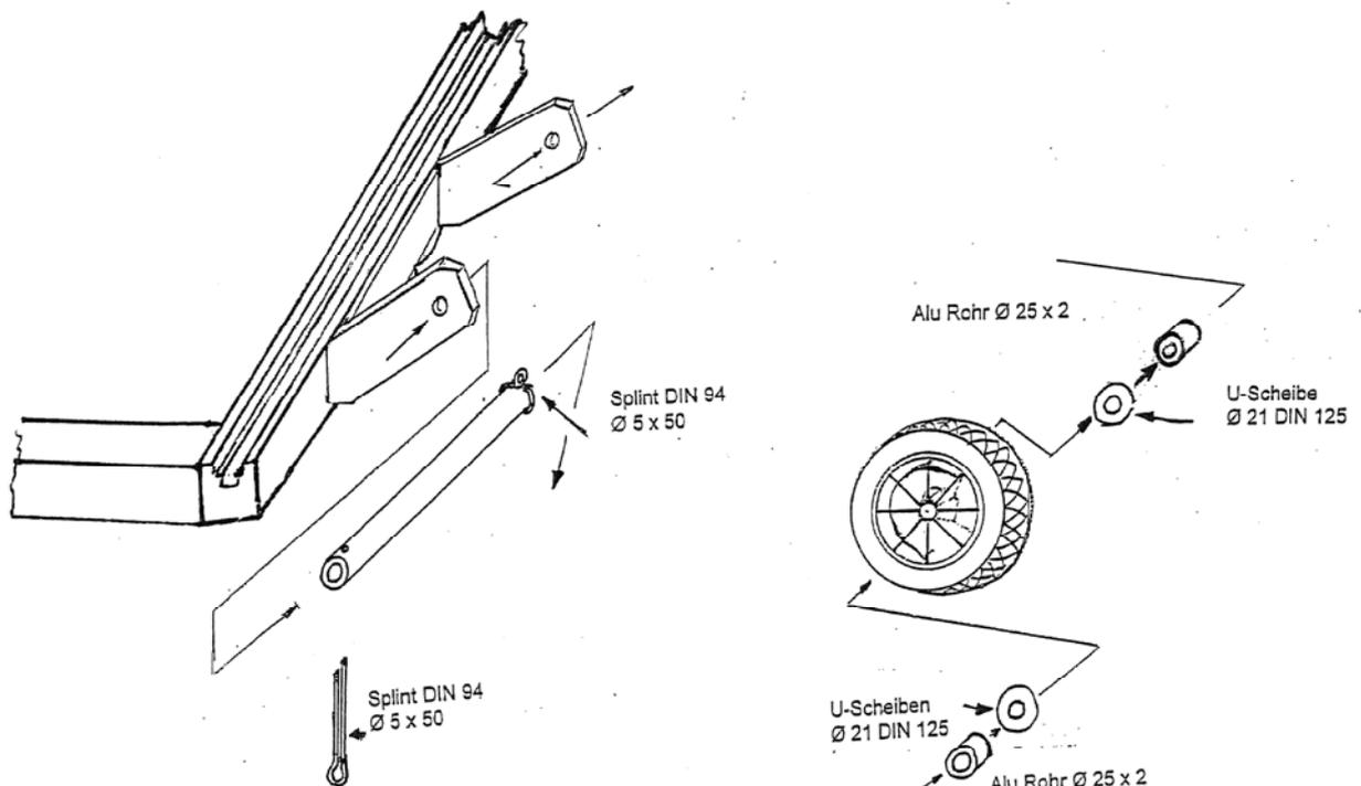
1. Mount the Wheels as shown on the drawing below.
