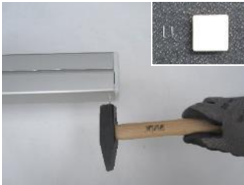
Fixing of cap in square upright:
