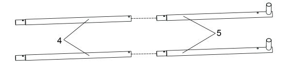
4. EN: Slip the step 3 assemblies into the side sleeves on the Net(19) as shown. Insert the Front Side Posts(4) into the Top Left Bent Tube(1) and Top Right Bent Tube(3) until the button snap into place as shown.
