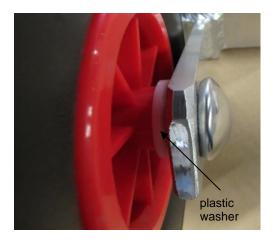
Finally hit 1 axle cap onto the wheel axle with a rubber mallet.
