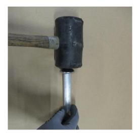
Hit the axle cap onto 1 wheel axle with a rubber mallet.
