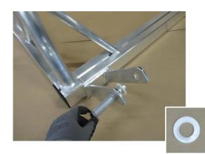
Insert the wheel axle from the outside through the hole in the wheel holder.
