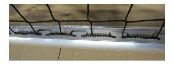
b) Now the tensioning rope can be knotted in the ring nuts mounted in point 2d).
