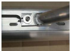
d) Stick from the inside ring nuts M6 x 50 for tensioning net rope through the open boreholes of both net hoops and fix with washers DIN 9021, 7.4 x 22mm and cap nuts DIN 986, M6.
