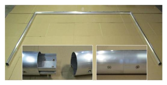
b) Turn the complete goal frame so that the guide rail faces upwards. Place net hoops in the upper corners and at uprights above threaded holes in the guide rail and screw safety hexagon socket cylinder screws DIN 912, M 6 x 20 together with washers DIN 9021, 7.4 x 22 mm.
