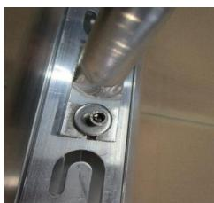
c) Place at both net hoops net hoop braces with rounded fitting above the bore hole in the net hoop and fix with hexagonal screw DIN 912 M6 x 40, washer DIN 9021, 7.4 x 22 mm und cap nut DIN 986, M6.
