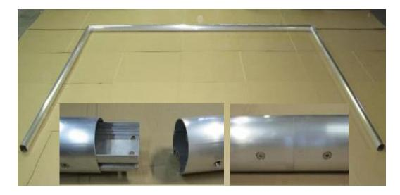
c) Set net hoops on both sides on the groove of upper corners and place nuts of point a) below holes of the welded fixing plates. 2 nuts each below the corner plate and 1 nut below the straight plate. Then stick washers DIN 9021, 7.4 x 22 mm on safety hexagon socket cylinder screws DIN 912, M 6 x 20 and screw net hoops in the nuts. Do not tighten them.
