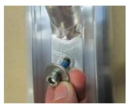
d) Place at both net hoops net hoop braces with rounded fitting above the bore hole in the net hoop and fix with hexagonal screw DIN 912 M6 x 40, washer DIN 9021, 7.4 x 22 mm und cap nut DIN 986, M6. To fix the net hoop braces at the crossbar push remaining nuts of point a) below the boreholes of the welded flat plates and screw hexagon socket cylinder screws DIN 912, M6 x 40 together with washers DIN 9021, 7.4 x 22
