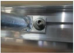
e) Adjust net hoops and net hoop braces and tighten all screwed fastenings.
