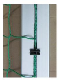
Pull the cord through each net meshes and fix it on both net hoops, if necessary lead it through the bore in the net hoop.
