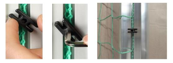
Pull the cord through each net meshes and fix it on both net hoops, if necessary lead it through the bore in the net hoop.
