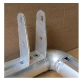
c) To fix the lower hinge stick from the bottom (upright's end) 1 nut 20 mm, M 8 each in the guide rail of the upright. Mount lower hinge with 1 fastening borehole. <u>Please consider that the inclined side of the hinge</u> <u>points to the goal inside</u>. Push nut 20 mm, M 8 below the borehole of the hinge and fix it at the upright with safety hexagon socket screw DIN 7991, M 8 x 16.
