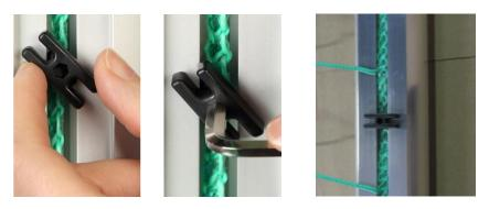
Cut the attached cord in half so that there are 2 short cords. Pull the cord through each net meshes and fix it on both net hoops, if necessary lead it through the bore in the net hoop.
