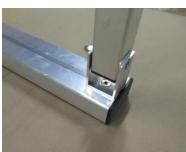
i) Press net hoop to the outside. Stick <u>from the</u> <u>top</u> hexagon screw DIN 933, M8 x 60mm through the 2<sup>nd</sup> borehole of the upper hinge and the hoop. Then add washer DIN 125, Ø 8.4 mm at the hinge lower side and screw wing nut DIN 315, M8.
