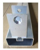
d) Beat cap 80 x 40 into the upright (use a mallet if necessary), adjust lower hinge and tighten fixing screw. Take care that the hinge at the bottom is flush with the upright's cap.
