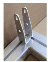
c) To fix the lower hinge stick from the bottom (upright's end) 1 nut 20mm, M8 each in the guide rail of the upright. Mount lower hinge with 1 fastening borehole. Please consider that the inclined side of the hinge points to the goal inside. Push nut 20mm, M8 below the borehole of the hinge and fix it at the upright with safety hexagon socket screw DIN 7991, M8 x 16mm.
