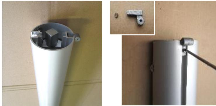
Fix cap at the support with 1 slotted pan head screw DIN 84, M4 x 40mm and self-locking nut DIN 985, M4. If necessary adjust support again and tighten grub screw.
