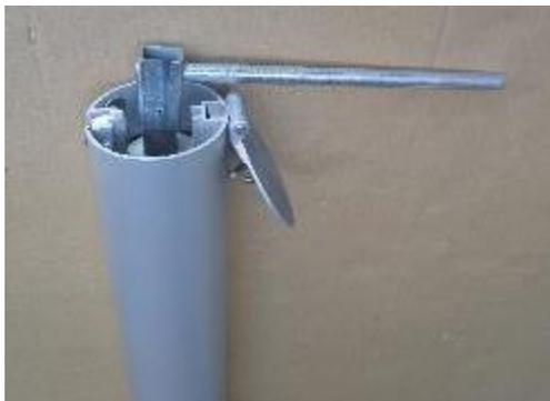
Open the cap at the mechanical upright and set the square key wrench on the spigot of the spindle. Now pull up the rope hook by turning the wrench.
