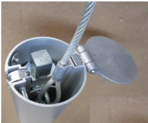
Pull the tensioning rope over the guide roller and fix it in the rope hook.
