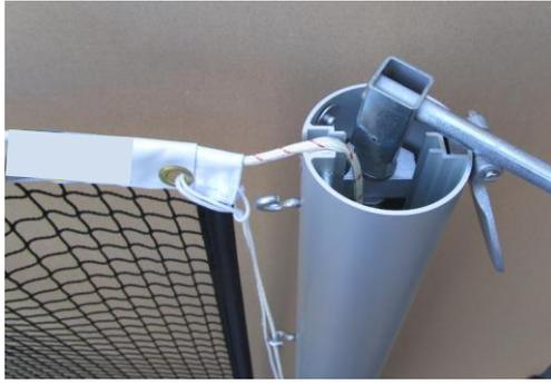
Then pull the hook down with the help of the wrench up to the requested net tension. If there isn't enough tension please consider the following point c).
