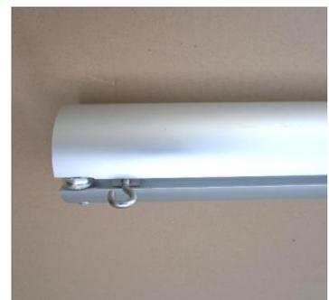
Turn the upright so that the opposite groove faces upwards. Push cap support into the groove and fix it slightly with 1 grub screw DIN 553, M6 x 8 mm.
